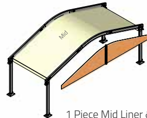
1 Piece Mid Liner & 2 Piece Gable Liner
